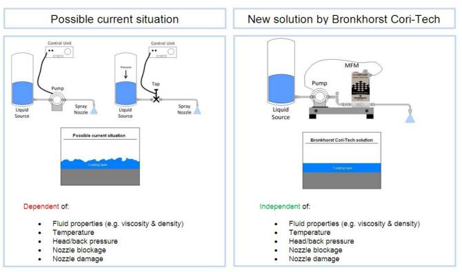
Bronkhorst Cori-Tech combines pumps with Coriolis meters. The pumps are directly (speed) controlled by the Coriolis instruments with integrated PID-controller, thus creating a mass flow pump with many advantages.
