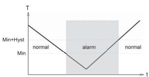
With a minimum-switch, falling below the limit value causes a switchover to the alarm state. Return to the normal state occurs when the limit value plus the set hysteresis is once more exceeded. With a maximum-switch, exceeding the limit value causes a switchover to the alarm state. Return to the normal state occurs when the measured value once more falls below the limit value minus the set hysteresis.
