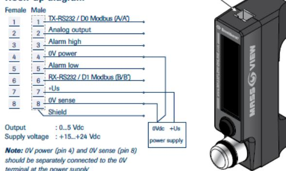
**Note:** 0V power (pin 4) and 0V sense (pin 8) should be separately connected to the 0V terminal at the power supply
