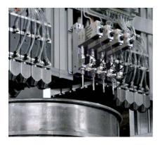
Dosing modules are available to dose liquid additives from rates as low as 0.1g/hr up to 500kg/hr
